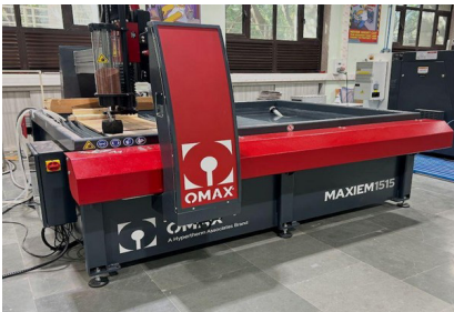
Abrasive Water Jet Cutting
